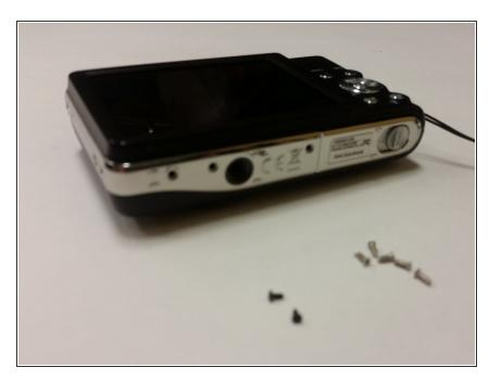
Remove the six 3 mm external screws from the camera base using the Phillips #000 screwdriver.
