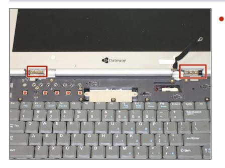
Using the Phillips #0 screwdriver, remove six screws that hold the LCD to the hinge.
