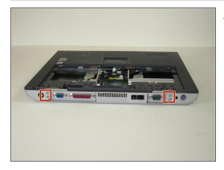
• Remove the four screws from the back of the case.
