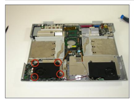
• Remove 4 screws holding left speaker for ease of access to connectors and external sound board.
