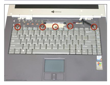
• Remove the 5 screws holding the keyboard in place.
