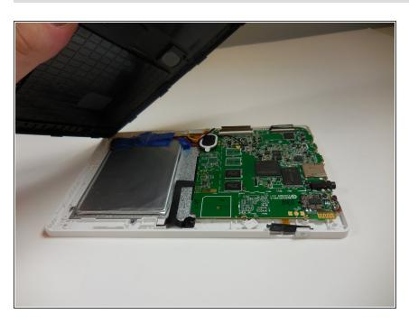
Use fingers to pry the rest of the back off; slowly apply pressure from each side to break each clip connection.
