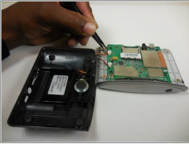
• Using the tweezers separate the wires connecting the battery and speaker to the mother board.
