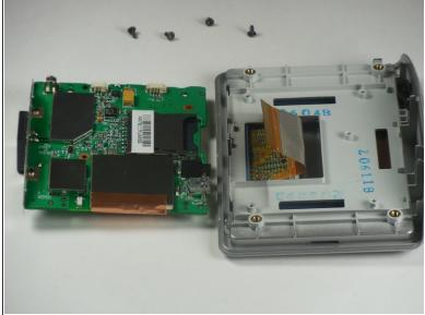
Detach the ribbon wire from it's port on the back of the motherboard.
