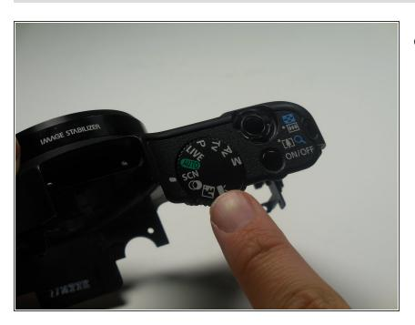
Locate and replace the format wheel on the front panel of the camera.
