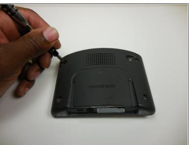
Remove the 4 .4mm screws on the back of the device.
