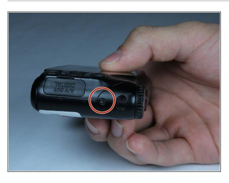
Remove the 5.0 mm black screw on the right with a Phillips #00 screwdriver.
