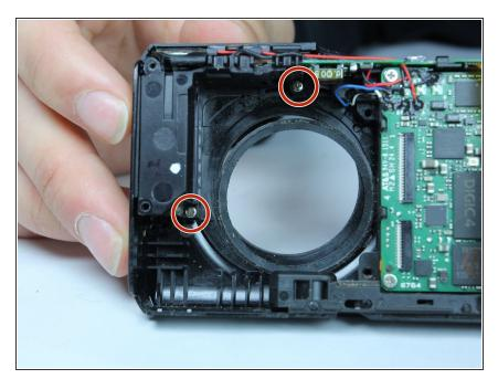
Remove the two 4.4 mm screws shown with a Phillips #00 screwdriver.
