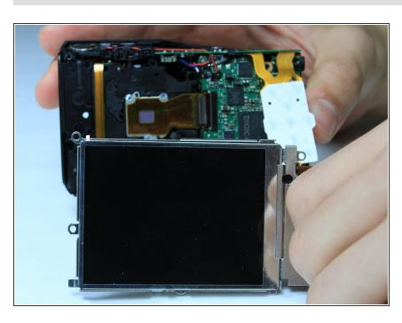
Holding the outer frame of the LCD screen, gently lift the LCD screen for replacement.
