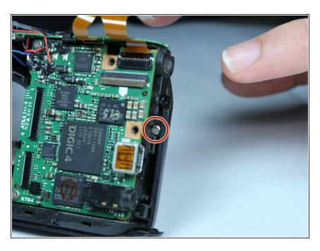
Remove the 4.4 mm screw shown with a Phillips #00 screwdriver.
