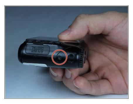
Remove the 5.0 mm black screw on the right with a Phillips #00 screwdriver.
