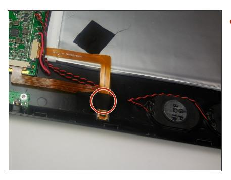
Remove the tape covering the ribbon cables and remove the camera module.
