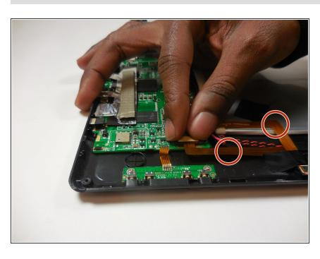
Remove the two ribbon cables attached to the logic board.
