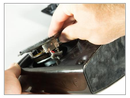
• You will notice 2 coils of wire around the speaker's input tabs. Slide these coils off as un-winding the wires may break the wires. Slide the coils around your new driver.
