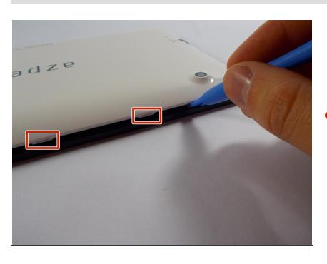
Next, gently pry the cover off with a plastic opening tool or a similar instrument by loosening all of the anchoring points. Two of the anchoring points are circled in the image. Avoid excessive bending or pivoting, since doing so may break the anchoring points.
