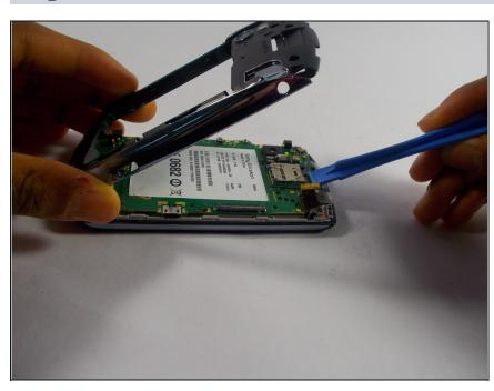
Separate the back cover from the phone. A plastic removal tool can be used here.
