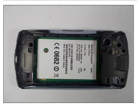
• Follow the Prerequisite Guide on how to Replace the Battery to prepare the phone for disassemble. Remove, but do not replace the battery.
