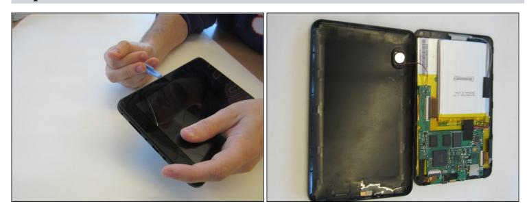
• Remove back cover with plastic opening tool, exposing the battery and motherboard.
