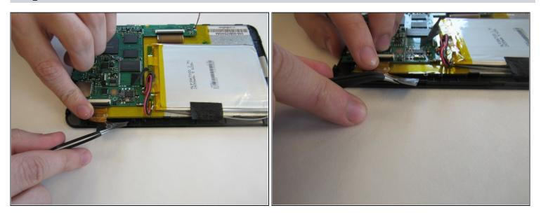
• Using the <u>tweezers</u>, remove the black tape connecting the screen to the motherboard.
