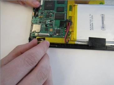
• Pull up the switch to remove the input connector.
