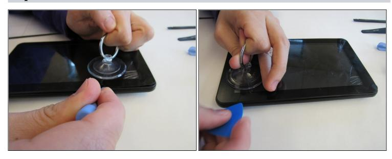
• Use the suction cup and plastic opening tool to pry the front screen from the tablet.
