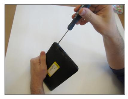
Remove two 2.4mm x 4mm screws from bottom of the tablet with Phillips #00 Screwdriver.
