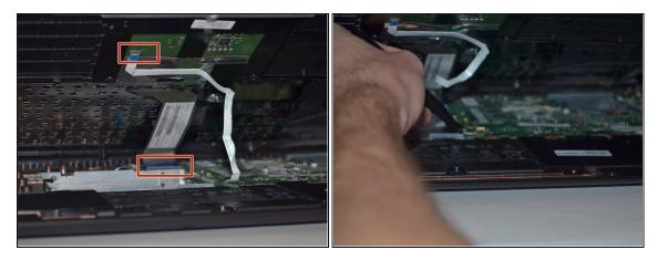
• Lift palm rest and unplug keyboard cable and touchpad cable using tweezers. After these two cables have been unplugged you can remove the keyboard cover panel.
