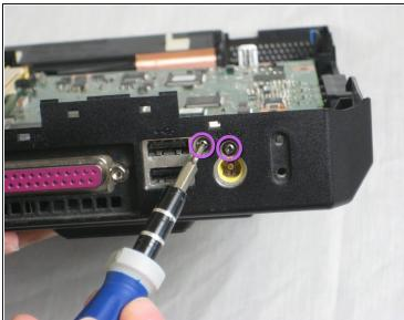
Remove the three 5.8mm screws with a Phillips #0 screwdriver.
