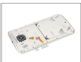
Twist off the screw and pry up the securing bracket.
