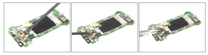
Release the connector and remove the rear camera.
