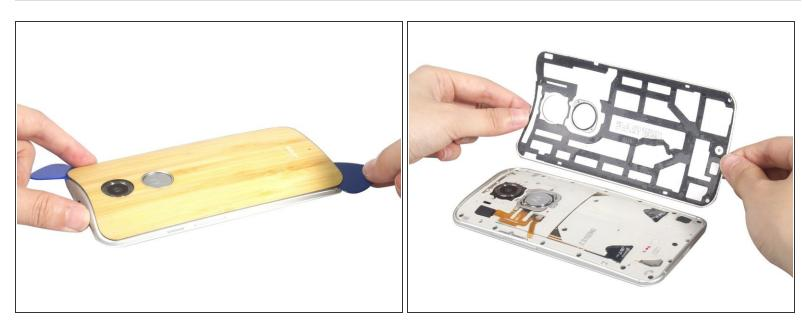
Slide the guitar pick to cut the adhesive sticker under the cover. It's a little strong. Finally, peel off the soft back cover.
