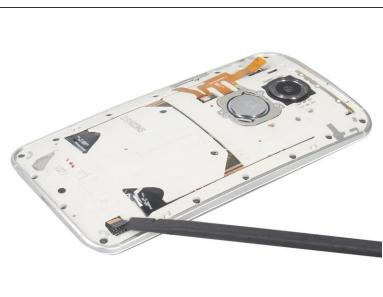
Release the side button flex connector and battery connector respectively under the rubber cover.
