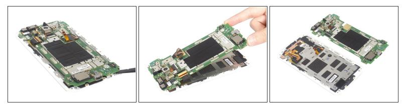
Pry up the motherboard and remove it carefully. At that time, we can separate the LCD screen from motherboard and get it alone.
