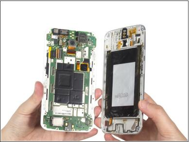
Twist off all 18 screws on the middle housing and remove it easily.
