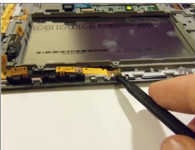
Release the button flex cable using the plastic spudger tool.
