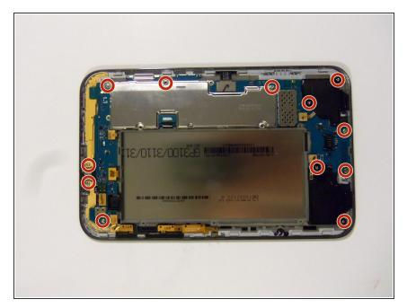
Using the Phillips #00 precisions screwdriver, remove the 12 4mm screws holding in the motherboard.
