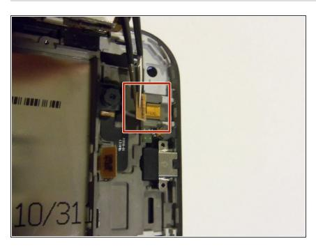
Remove the front facing camera using the precision tweezers.
