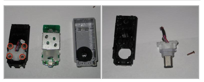
• Remove four tri-wing screws to remove the connector from the housing.
