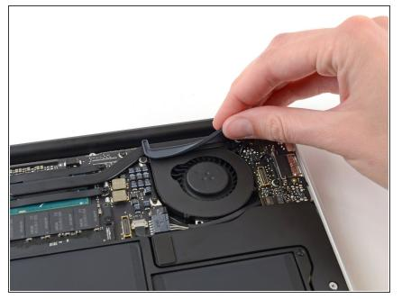
• Peel the rubber gasket off the adhesive on the top of the fan.
