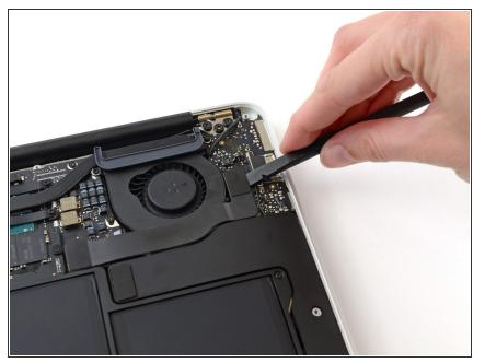
Use the flat end of a spudger to pry the I/O board cable connector up out of its socket on the I/O board.
