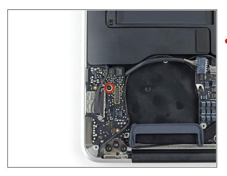
Remove the single 4.1 mm T5 Torx screw securing the I/O board to the upper case.
