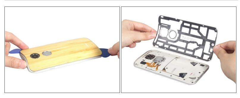
Slide the guitar pick to cut the adhesive sticker and peel off the soft back cover.
