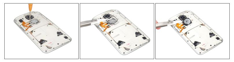
Twist off three screws, pry up the securing bracket and remove the logo finally.
