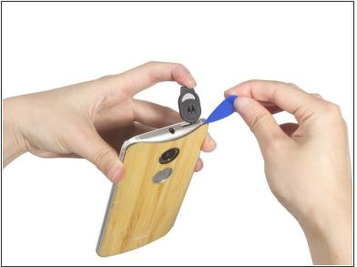
• Use the eject pin to open a gap and place a guitar pick into the gap.
