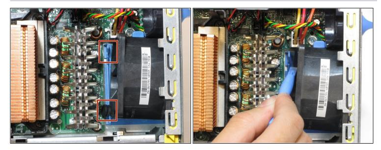
Remove the rubber grommets from the base of the fan. The iFixit Opening tool may be useful in this step.
