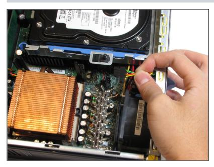
Remove the power supply by pressing the release tab. It is distinguished by the black, red, green, and yellow wires.
