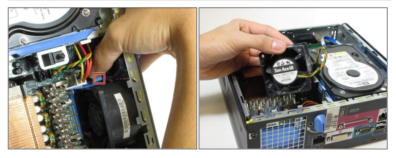
• Press on the blue release tab and remove the fan.
