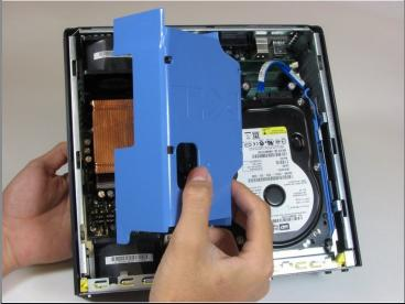
Remove the large blue cover from the computer. There are no screws or tabs holding it in place.
