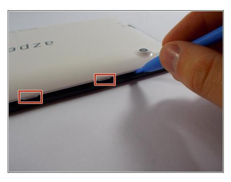
Next, gently pry the cover off with a plastic opening tool or a similar instrument by loosening all of the anchoring points. Two of the anchoring points are circled in the image. Avoid excessive bending or pivoting, since doing so may break the anchoring points.
