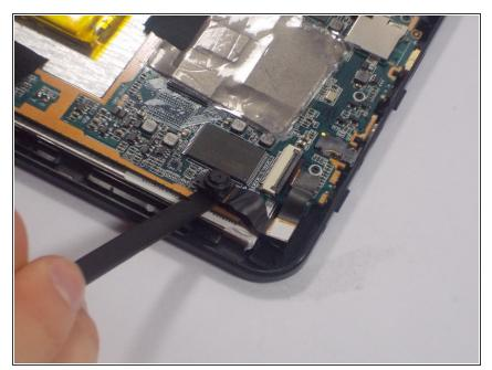
Using the spudger, pry the rear facing camera its power strip off the circuit board. This may require some force, since a strong adhesive is used to mount the camera assembly to that point.
