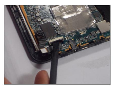
Lift open the connector flap with the spudger.
