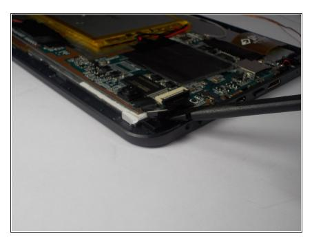
Gently pull the front facing camera out of its mounting point. Use a spudger if necessary.
