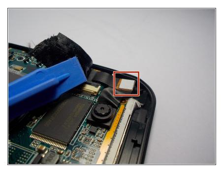
Using a plastic opening tool, gently peel back the black electrical tape to reveal the power strip and the front facing camera, which is marked by the red box in the image.
