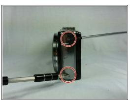
Take a Phillips Head screwdriver and remove the 2mm screws on the left and right side of the camera.
