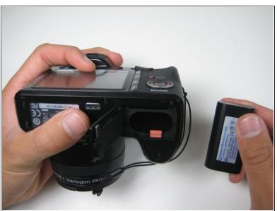
Once the battery has popped out of the compartment, simply pull it out of the camera.
