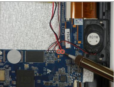
Carefully desolder the 2 wires that connect the battery to the motherboard.
