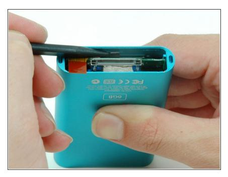
Use a spudger to pull back on the small black plastic tab holding the click wheel in place.
