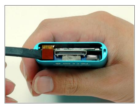
Use a spudger or the tip of your finger to carefully disconect the orange click wheel ribbon from the logic board.
