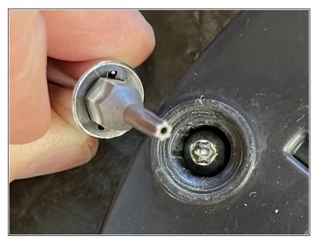
Also the front two screws are safety screws: they have a 6 sided star shape with a raised dimple in the center to prevent homebodies from casually opening the machine. (probably from the Sunbeam's (owns Mr. Coffee) legal dept.)
