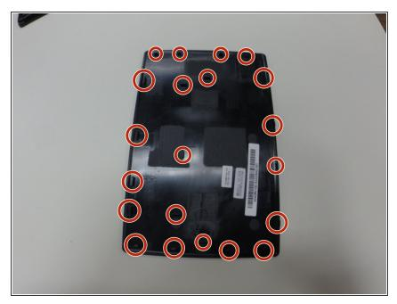
During Reassembly this is where the plastic snaps are located on the back cover. They will have to be lined up in order for it to snap back into place correctly.
