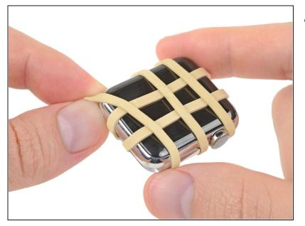
• For best results, detach the watch band and wrap a couple rubber bands around the Apple Watch's case to help the adhesive bond correctly.
