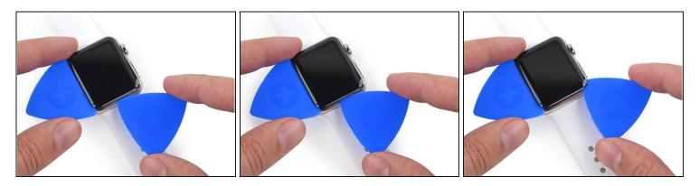
• While holding the first pick in place, use a second to check that all of the adhesive is separated around the entire perimeter of the screen.
