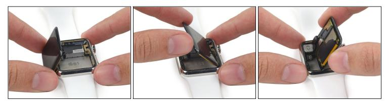
• Fold the screen up and over to the right, to expose the cables underneath.
