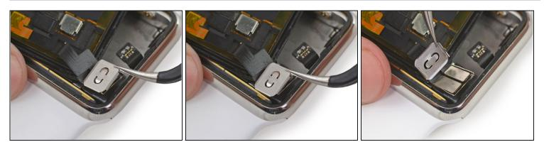
• Grab the cover with your tweezers and slide it toward the top of the watch to free the final slotted tab, and remove the cover.
