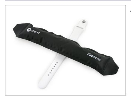
Microwave your iOpener for another 30 seconds, and apply it to the front of the watch case to soften the adhesive securing the Force Touch sensor.
