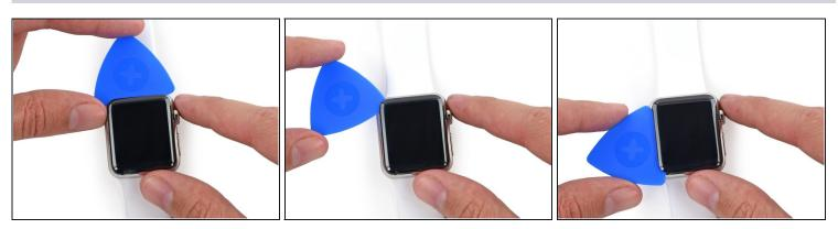
• Continue working the pick around the perimeter of the screen, rolling down along the left side to cut the last of the adhesive.
