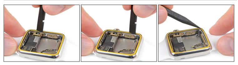
• Gently but firmly press the Force Touch sensor into place all around the perimeter of the watch case.
