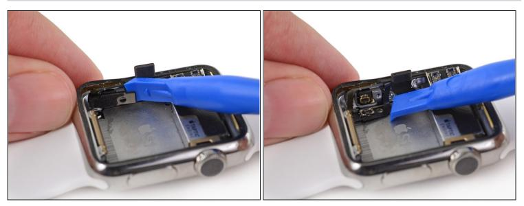
• Use a plastic opening tool to flip the Force Touch sensor cable connector straight down, disconnecting it.
