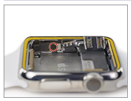
Replace the Y000 tri-point screw securing the Force Touch sensor connector cable.
