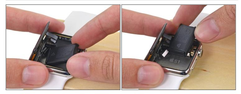
• Rotate the battery counterclockwise to expose its connector.
