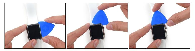
• Work the pick around the top right corner, and roll it along the top edge of the screen.
