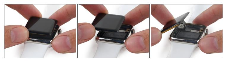
• Lift the screen up and shift it to the left, minding the display data and digitizer cables.
