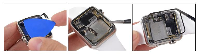
• Use a plastic opening pick and <u>tweezers</u> to remove the Force Touch sensor from the case.
