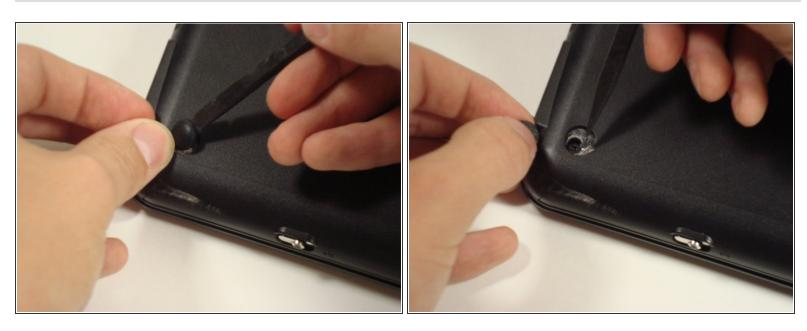
Remove the rubber pads located on the corners of your Compaq Mini.
