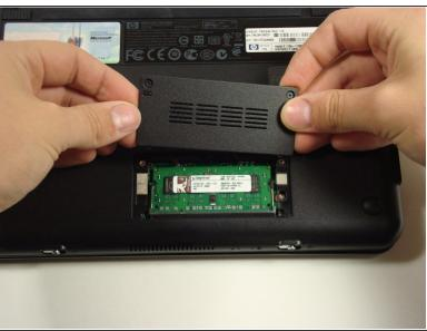
Use a Philips #0 screwdriver to unscrew the two screws covering the memory compartment on the bottom of the laptop and remove the cover.
