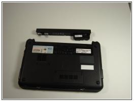
• Push both tabs inward simultaneously and slide the battery out.
