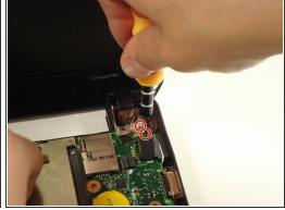
Remove the four screws that keep the bottom of the hinges attached to the base.
