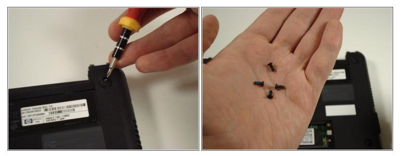
• Unscrew all the corner screws. There are four total, one under each rubber pad.
