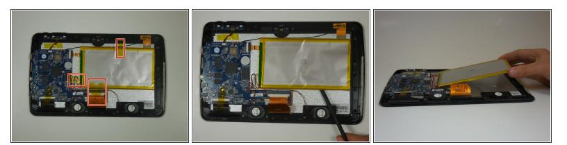
• Use a spudger to carefully remove the tape nearest to the battery.
