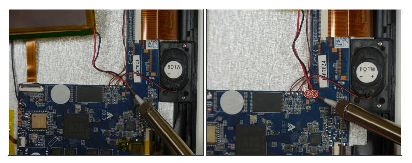
• Carefully desolder the 2 wires that connect the battery to the motherboard.
