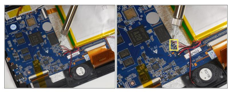
Carefully desolder the 4 connections of the speakers.
