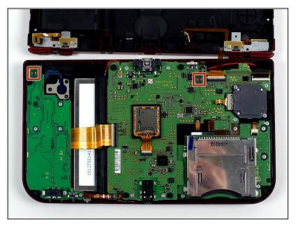
Use a pair of tweezers to lift away the two plugs that latch the L/R/ZL/ZR button ribbons to the motherboard. You can now remove the back cover completely and set it aside.
