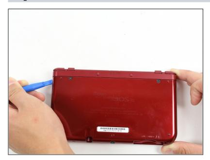
Once the screws are loosened, pry open the back cover.
