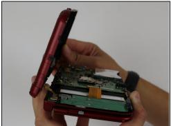
• To separate the cover, carefully lift it up and away from the hinges (in order to clear the headphone port), then pivot it towards the hinges to expose the circuit boards.
