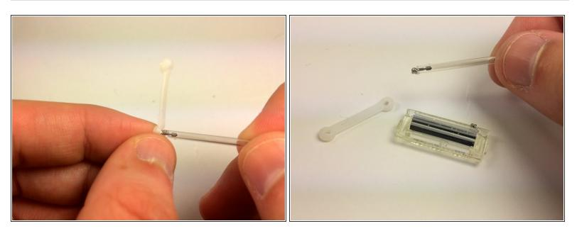
• Completely remove the rubber band from the flash bulb.
