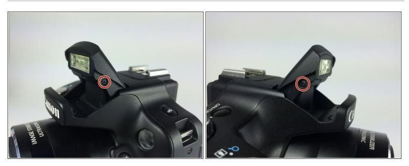
• Remove the two Phillips #000 screws, length 3 mm, on both sides of the flash.
