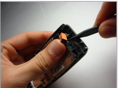
With the logic board and LCD unit removed, gently pry out the vibrator from its housing.
