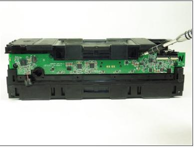
• Remove the four T6, 9.9mm screws that secure the button circuit board to the body
