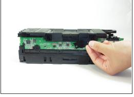
• Remove the two PH0, 5.8 mm screws on the small plastic black panel using a screwdriver.
