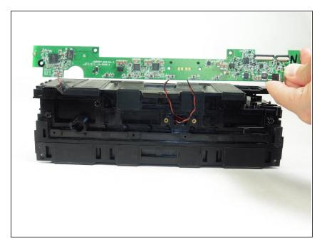
Minding the small L-shaped piece of metal on the end opposite of the ports, lift the circuit board from the body of the Big Jambox.
