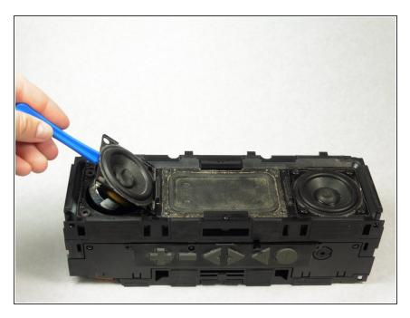
Using a plastic opening tool, pry the speaker out of the Jambox.
