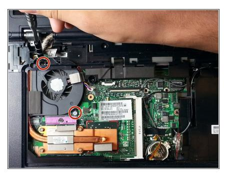
Using a Phillips #1 screwdriver, unscrew the two 7mm screws on the top and bottom of the fan.
