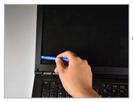
• Using the plastic opening tool, gently pry off the plastic LCD screen frame around the entire perimeter.
