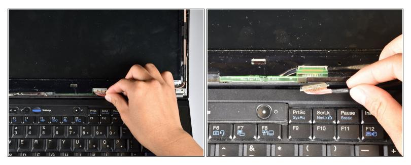
• Remove the LCD connector by pulling on the ribbon cable at the connection.
