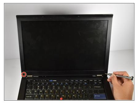
Use a #0 Phillips head screwdriver to remove the two 3mm screws that hold the screen bezel in place.
