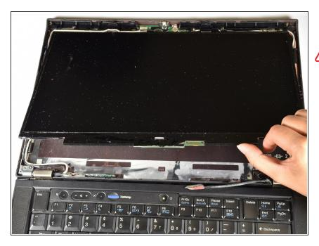
• Lift the LCD screen out to replace.
