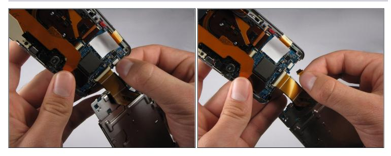
• Disconnect the small ribbon-wire by gently pulling on the small ribbon-wire where it connects with the motherboard.
