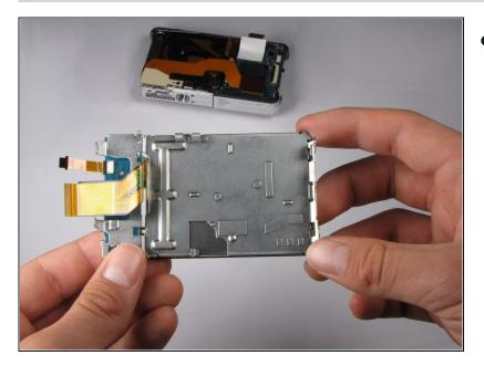
• Pull the LCD and its casing away from the rest of the camera.
