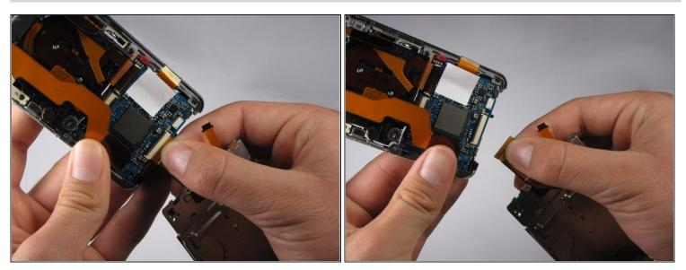
• Disconnect the large ribbon-wire by pulling on the large ribbon-wire where it connects to the motherboard.
