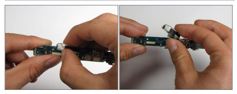
• Gently wiggle the flash bulb to remove it from the joints.
