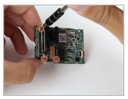
Using your screwdriver, remove the three 4mm PH00 screws that hold down the metal plate.
