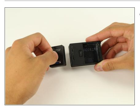
Use the battery tab to pull the battery out of the device.
