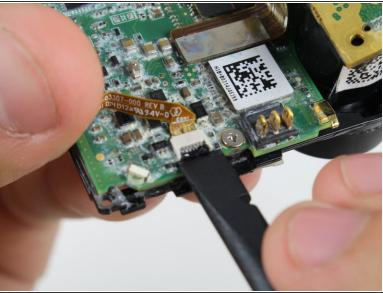
Remove the ribbon cable connecting the housing to the motherboard by flicking up the black clip with the spudger tool and gently pulling the cable out.
