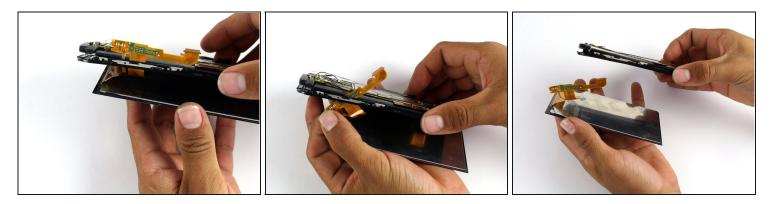
• Carefully guide the display assembly ribbon cable through the midframe for removal.
