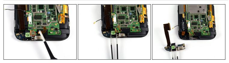
• Remove the single silver 4mm T5 Torx screw securing the headphone jack/micro USB board.
