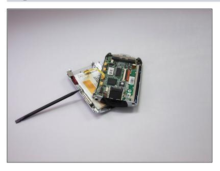
• Carefully remove the back cover using the spudger against the grooves along the sides of the iPAQ.
