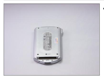
• To begin the disassembly of the device, place it on a flat surface with the screen facing down.
