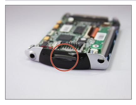
Remove SD card on top of device by pushing and then releasing.
