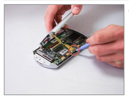
• At this point, a yellow ribbon will be connecting both the front and back panels of the device. Carefully use the plastic opening tool to detach the ribbon from the connector pins.
