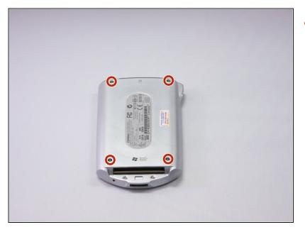
• Remove the four screws found on the back cover of the device.
