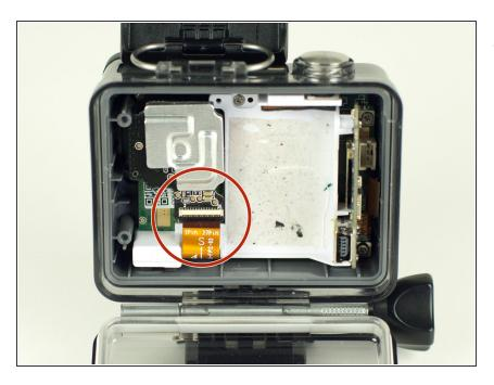
Disconnect the ribbon cable from the lens by lifting the black latch and gently pulling the ribbon cable from the socket.
