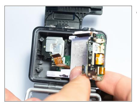
Carefully remove the motherboard and white plastic piece from the case.
