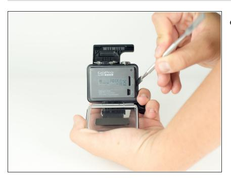
Gently pry the back open by inserting a metal spudger between the case and back panel.
