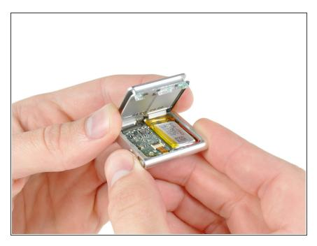
Remove the rear panel from the Shuffle.
