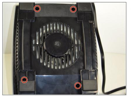
Use a screwdriver to remove the four screws that are next to the grip pads on the bottom of the motor base.
