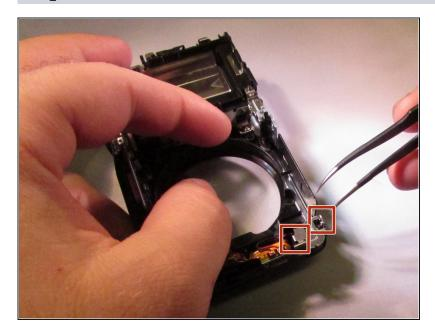
Use <u>tweezers</u> to remove the speaker retaining clip. The retaining hooks locations are indicated, but not exact.
