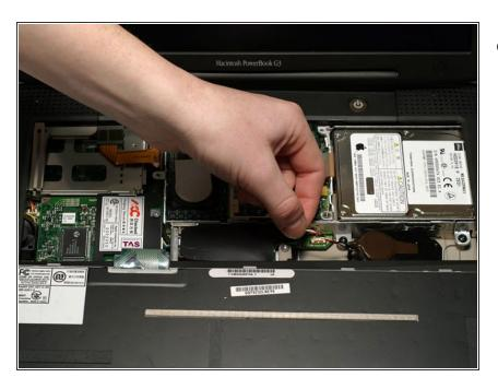
Remove the battery from its holder by pulling up and to the left.
